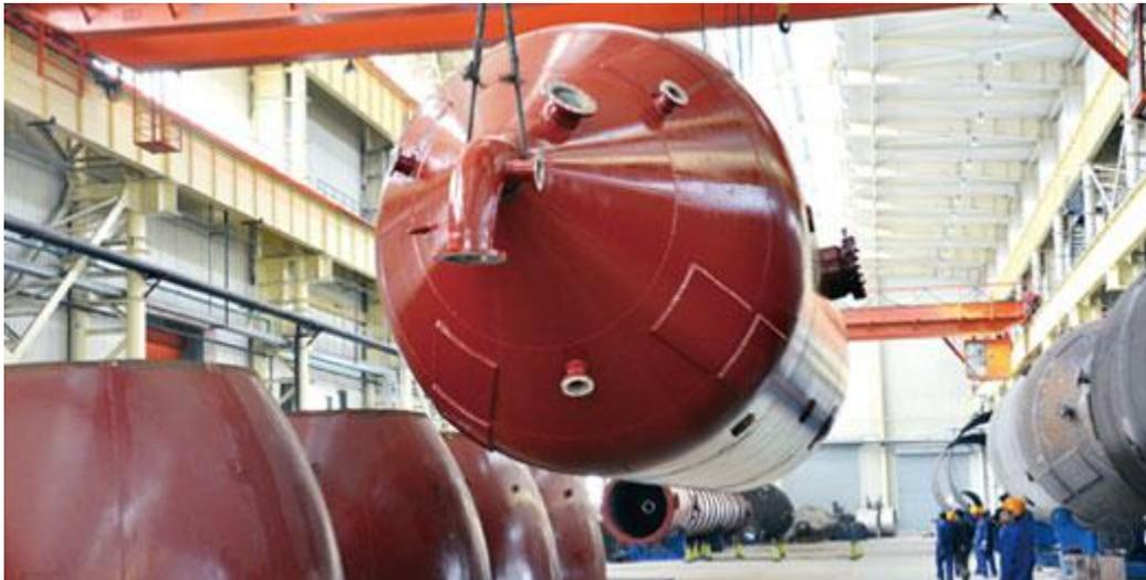
The maximum size of the pulping digester is 5.8m in diameter and 400m<sup>3</sup> in volume. Digester series are made of different raw materials including carbon steel, 316L steel, stainless steel and composite plate, duplex stainless steel structure. They are majorly used to chemical pulp and dissolved fiber steaming section.
