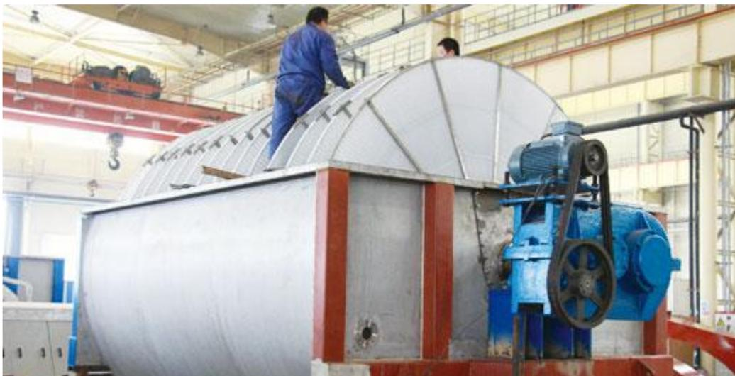
Disc filter can be used in various sectors with features such as large effective filtering area, easy to dismantle, and high strength etc.
